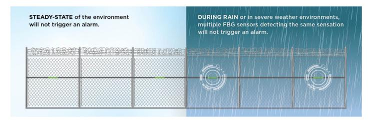
Coupled with adaptive thresholding, AGIL Fence PIDS consistently monitors inputs from each FBG sensor in real-time. It adapts the threshold for each sensor automatically and dynamically in reference to the environmental conditions such as strong winds, heavy rains and sand storms affecting that sensor. Advanced Signal Processing collects and processes data to differentiate and identify scenarios, even in extreme environments.
